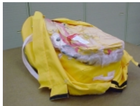
Packed carrying case including vacuum-packed raft and accessory kit container.
