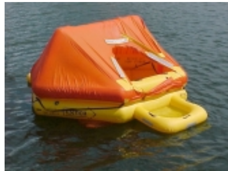
Deployed eight-person life raft. The twelve- and twenty-person rafts have the same design.
