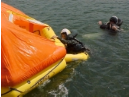
Two aircrew conducting boarding tests on the 8-person raft during Operational Testing at Naval Operational Medicine Institute, NAS Pensacola.
