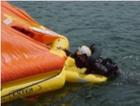
Female aircrew conducting boarding tests on the eight-person raft during Operational Testing at Naval Operational Medicine Institute, NAS Pensacola.
