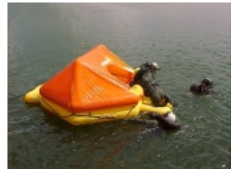
Four aircrew conducting boarding tests on the 8-person raft during Operational Testing at Naval Operational Medicine Institute, NAS Pensacola.
