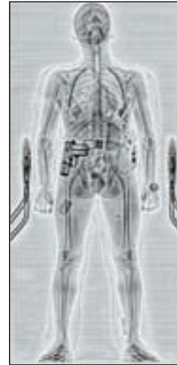
FIGURE 5. Transmission X-Ray Image of a Person with Threat Objects
