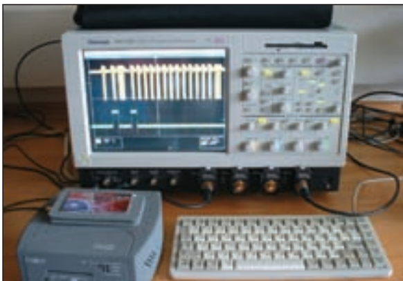
FIGURE 3. Noninvasive Counterfeit Detection Using Waveform Measurements
