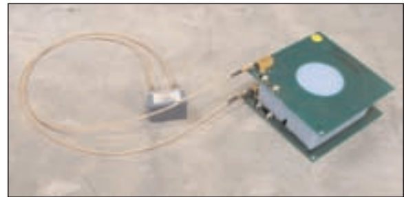
FIGURE 1. Dual Loop Antenna Used for Jamming Research
